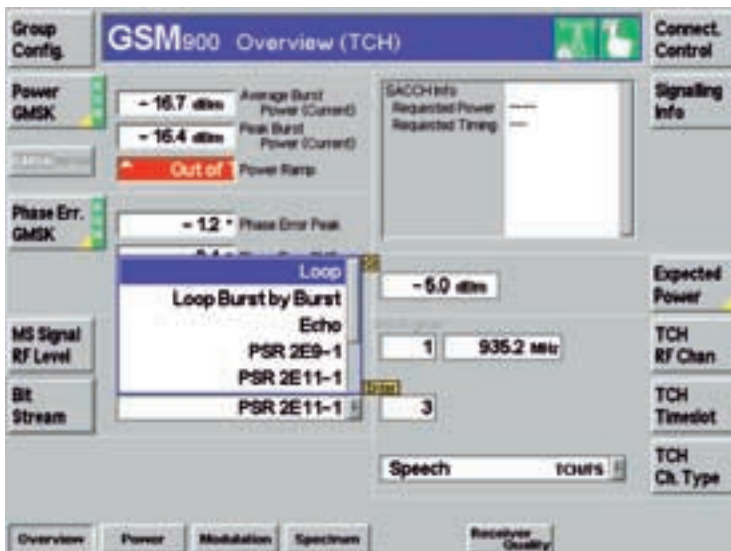
FIG 2 For bit-error-rate measurements, a bit sequence can be selected from a list, or CMU 300 itself can be used as an RF loop if the DUT sends the data stream
