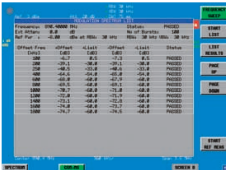
FIG 4 Display of results measured for spectrum due to modulation
